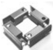
Slot and Tab (Self-fixturing)
