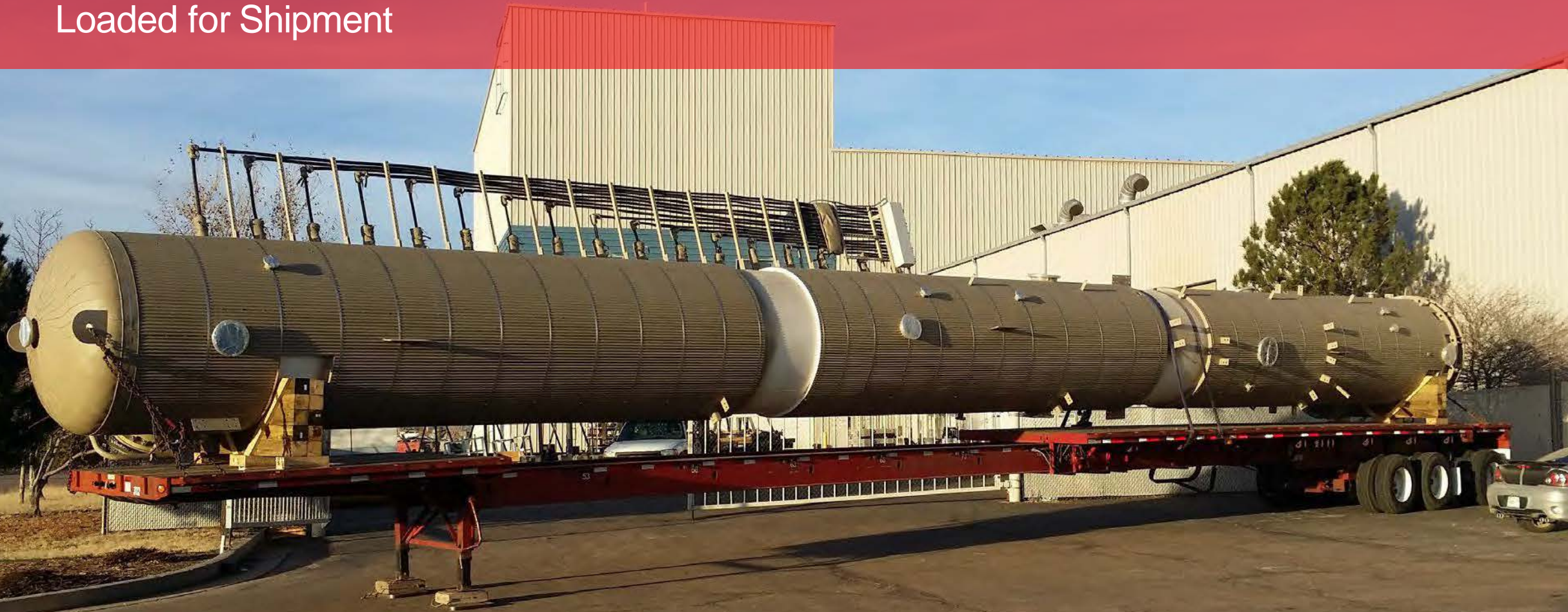
Stabilizer Tower 6ft x 82ft / Anadarko Petroleum Corp.
